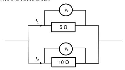
What is the reading on  $V_1$  if the reading on  $V_2$  is x V?
