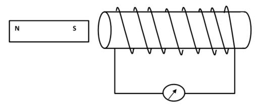
The magnet is now pulled out of the solenoid with a greater speed as before. The galvanometer needle will deflect ...
